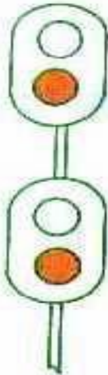
Warner 'ON' Position Outer 'ON' Position
